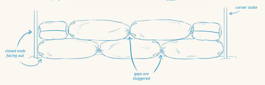
This process repeats for each course. Be sure to check for plumb using a level or a weighted line as you move along. You want to make sure each wall is perfectly vertical. Any slight lean as you build will continue to get worse as the wall gets higher. To help tie the structure together vertically, the Tetrad crew cut pieces of steel rebar into 4-6 ft. lengths and drove them down through the bags with a sledgehammer. The ends of the rebar
