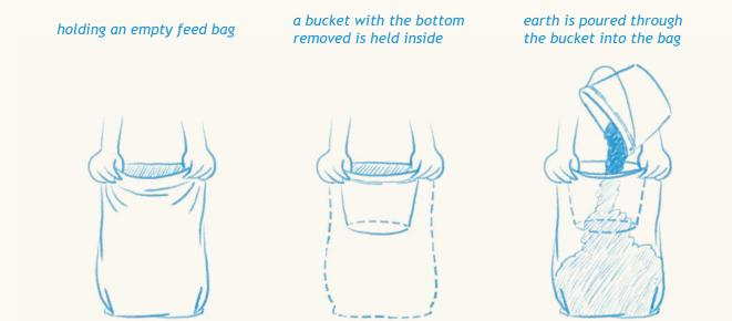
Before filling, the bottom of the feed bag was positioned exactly where it was needed on the wall. Once all 4 buckets were in the bag, the top of the bag was folded over 3-4 times creating a 2" flap that was stapled shut. The bag was then lowered squarely into position on the wall.
